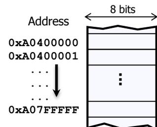
As per the figure, we only need 22 bits for the address in the given range (where the memory device is located). Thus, the size of the memory device is  $2^{22} = 4\text{MB}$ .
